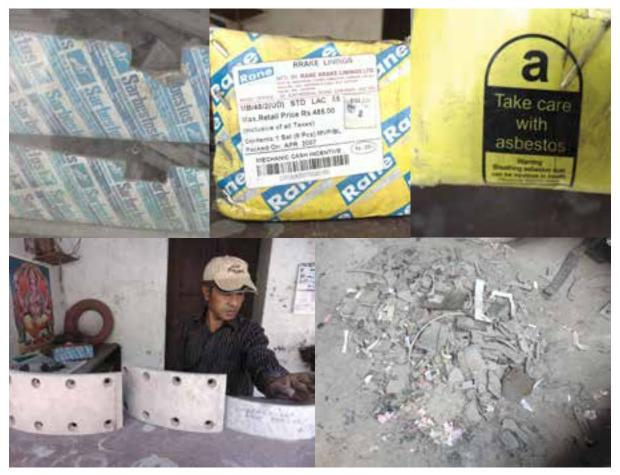
Figure 11. Pictures of Asbestos lining Materials, Worker and Waste at Working station, Putalisadak, Kathmandu
